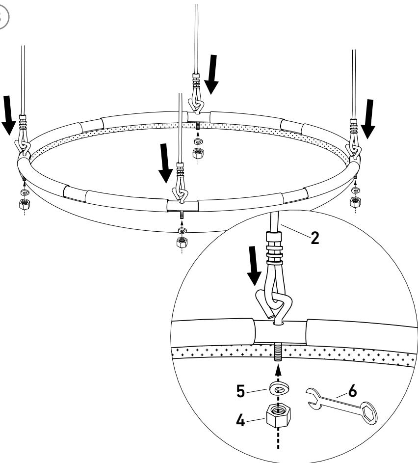
**NOTE!** Pass the screw with the eyelet down through the swing until the threaded part of the screw protrudes below. Then securely screw parts **5** and **4** in place (see picture above) using the wrench.
